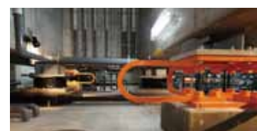
Layer Rubber Isolator and Integrated Layered U-type Damper
